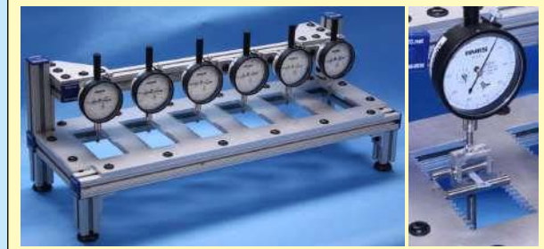
Figure 9 - three-point bend test fixture for long term creep testing
